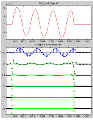
Fig.13 Wavelets Coefficients of External Faulty Signal
